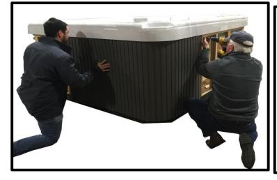
With a helper continue wrapping panel around spa keeping enough tension on panel to eliminate any buckling. Fasten panel into bracing using three of the provided screws in the top, middle, and bottom of the panel
