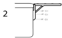
Secure each roller rack to the spa skirt by inserting all six #10 screws tightly into the screw holes that you marked in the previous step.
