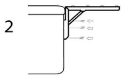
Secure each roller rack to the spa skirt by inserting all six #10 screws tightly into the screw holes that you marked in the previous step.
