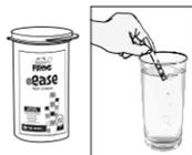
**b.** Look at the **Total Alkalinity** reading first. Adjustments should be made to bring the Total Alkalinity in the **range of 80 – 120 ppm** prior to making any adjustments to pH even if it throws pH off further.
